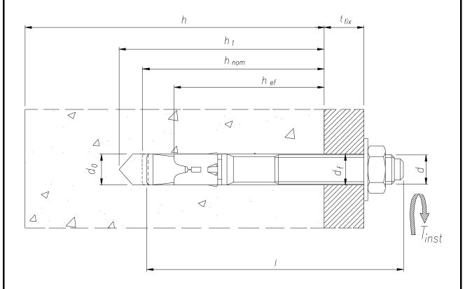
$\begin{array}{l} h_{ef} \colon \text{effective anchorage depth} \\ h_{nom} \colon \text{embedment depth} \\ h_1 \colon \text{drilling hole depth} \\ t_{fix} \colon \text{fixture thickness} \end{array}$
